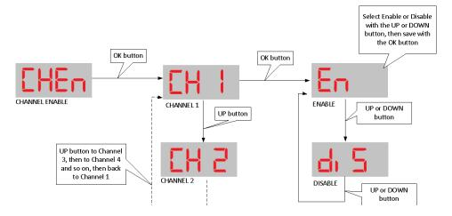
In this menu, you can enable or disable a channel from displaying a temperature. You might want to do this if a fiber optic probe was not hooked up (values for this channel do not apply) or if a probe was broken along the way and thus the displayed temperature is known to be incorrect.
