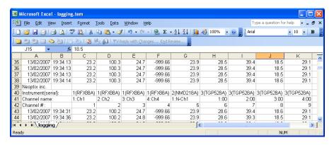
When logging temperatures for a very long time, one needs to note that a standard Excel sheet is limited to 65535 lines. If this limit is reached, the logging process will close the current data-logging file, and will open a new one, with the same name but with "\_1" appended to the file name, and so on ("\_2" ...), until the application is stopped or your disk becomes full.
