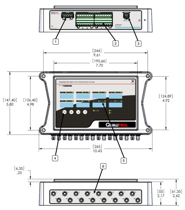
The following drawing, below, could be useful especially if you mount the unit on a swing panel, as it gives the details of the required cutout hole for such installation. Furthermore, details on the required bolts are given (M8).
