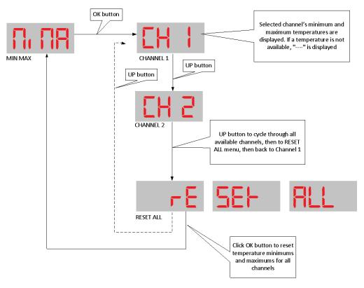
In this menu, you can view at a glance what the minimum and maximum temperatures measured were for each available channel.
