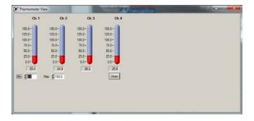
All thermometers share the same Min / Max reading setting. Refresh rate is fixed at 1.0 sec. The size of this window will change depending on the number of channels to display. Up to 16 thermometers can be shown; if you want to display more than 16 channels, only the first 16 detected channels will be shown (note that any channel that has its "Chart" checkbox unchecked, in the main window, will not be shown).
